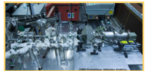
Analyseur FAKIR (Facility for Analyzing Krypton Isotopic Ratios)
